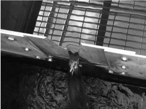
V notch weir: Typical 5/2 power law
