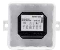
LET210 single-channel receiver – Can be fitted in a recessed junction box – Degree of protection IP55 (in the junction box) – 5 A (NC) or 10 A (NO) contacts – For four drives
